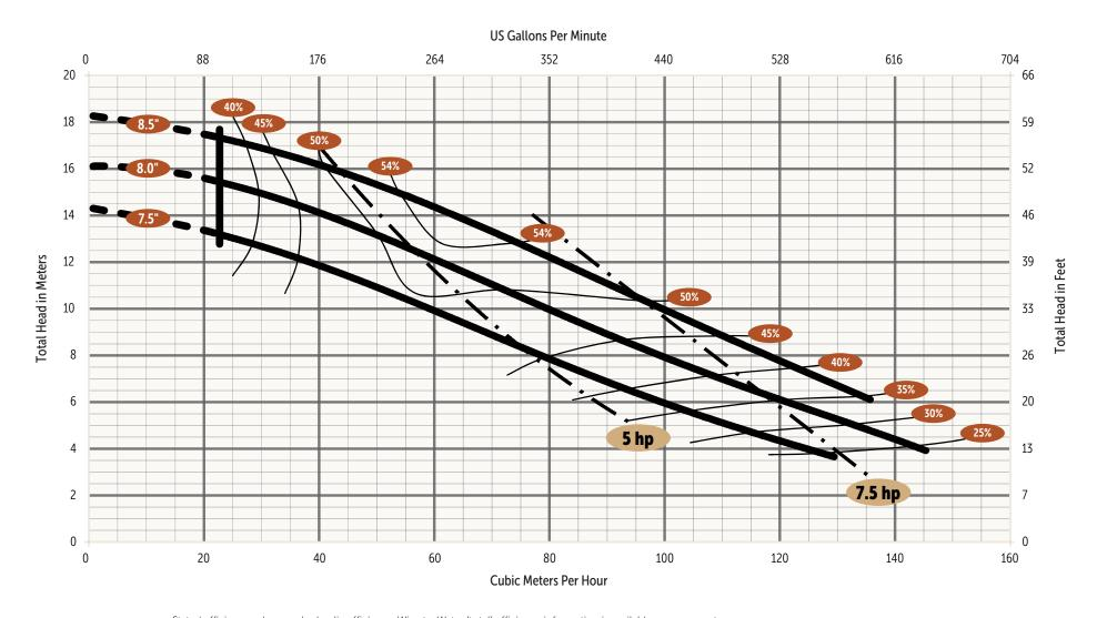
Stated efficiency values are hydraulic efficiency. Wire-to-Water (total) efficiency information is available upon request.
